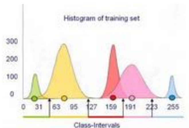
Figure 4.14: Classification using closest distance to the class mean
